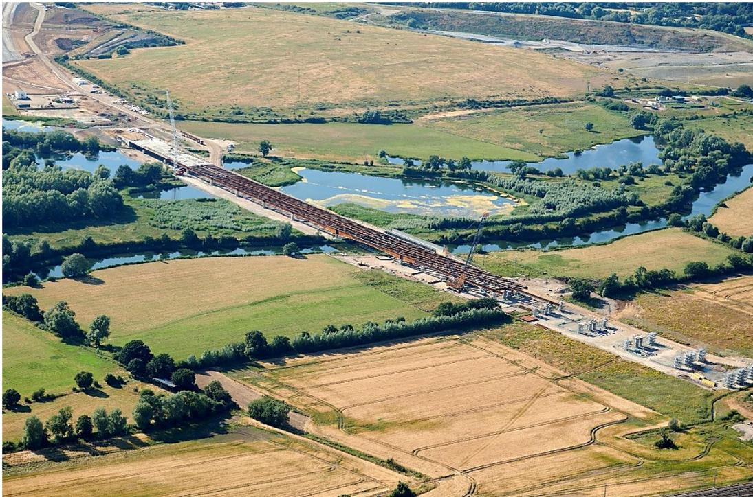
The bodies of water, visible from Brampton Road Bridge over the realigned A1 are essential to ensure that the highway drainage is separate from the existing land drainage systems.
